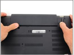
Slide the switch on the right side of the battery to the right while applying upward pressure on the battery.
