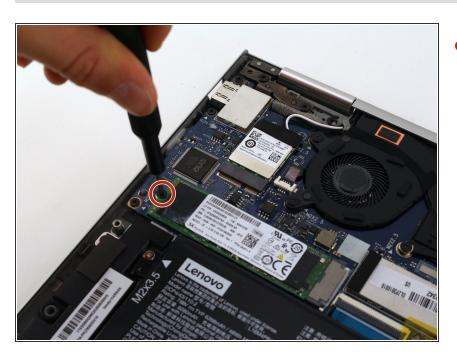
Use a Phillips #00 screwdriver to remove the 4mm screw holding down the storage drive.
