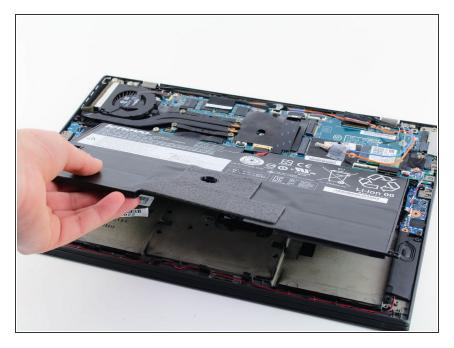
Remove the battery by pulling it directly towards you.
