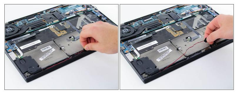
Remove the tape that is holding down the wire that connects the two speakers.
