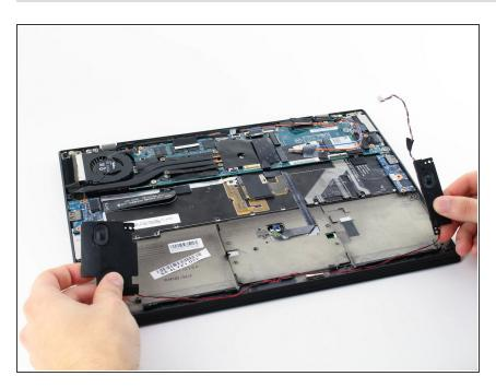
Remove the speakers by lifting them directly upward.
