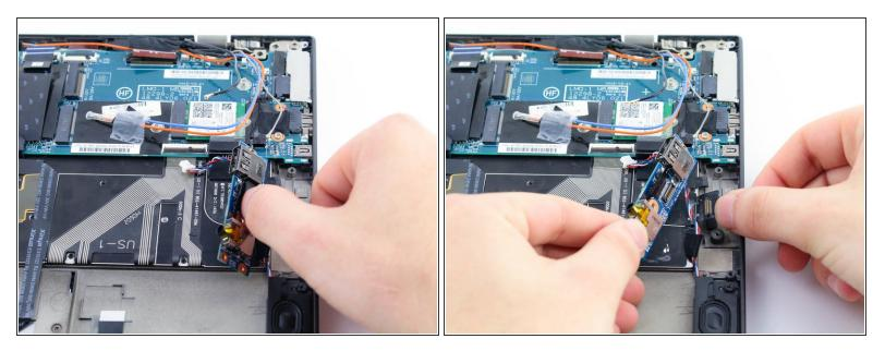
Undo the clasp under the USB audio port board.
