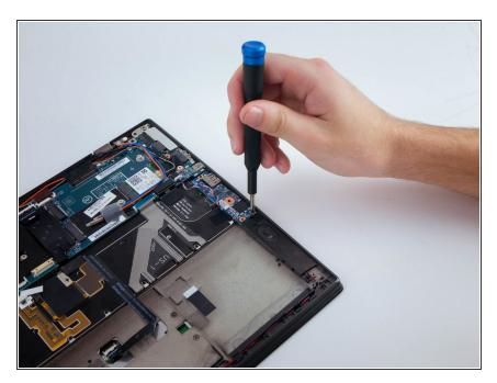
• Use a Phillips #0 screwdriver to remove the 2.9 mm screw that is holding down the USB audio port board.
