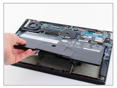
• Remove the battery by pulling it directly towards you.
