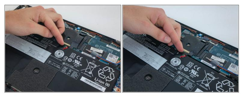
• Using your fingers, disconnect the battery from the motherboard.
