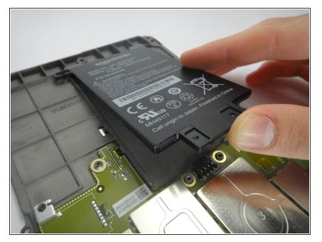
• Gently lift the battery from the bottom, and slide it out of the midframe.
