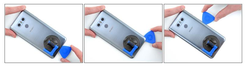
Re-insert the opening pick into the bottom edge of the phone and slide it up the right edge of the phone, cutting through the adhesive holding it in place.
