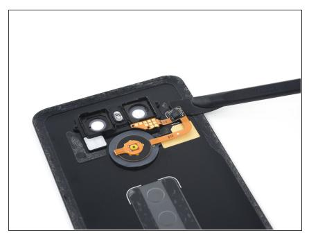
Use the blade of a halberd spudger or another plastic pry tool to pry the rear button chip off of the rear case.
