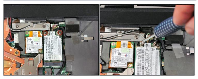
• Using a #0 Phillips screwdriver, remove the two 10.5 mm screws.
