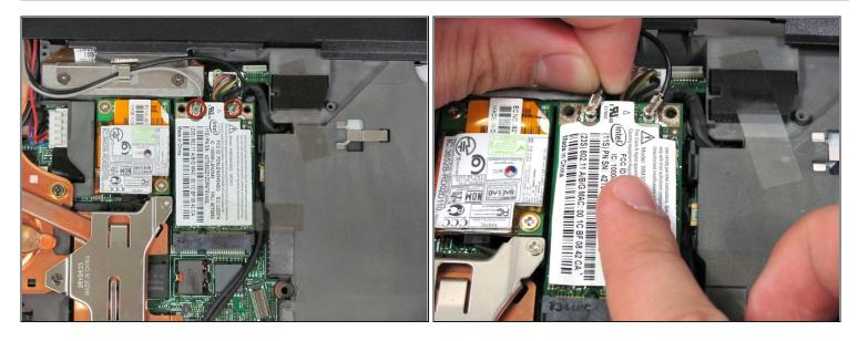
• Disconnect the two connectors by pulling upwards on the base of the grey and black cables.
