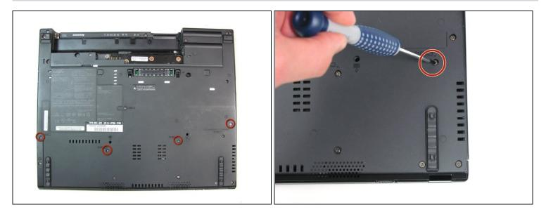
• Using a #0 Phillips screwdriver, remove the four 17.0 mm screws.
