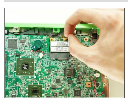
Gently remove the two antenna cables by lightly pulling the cable connectors up.
