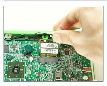
Remove the wireless card by gently lifting it out of the socket. To reassemble your device, follow these instructions in reverse order.
