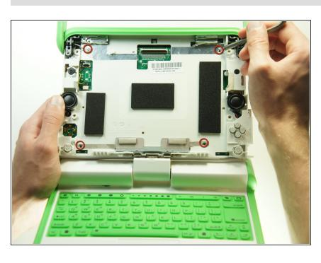
Remove the four 4mm Phillips #1 screws that hold the top cover to the case.
