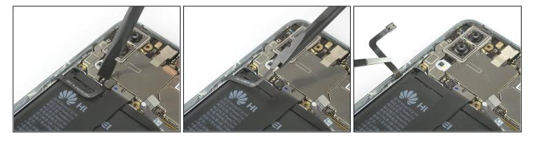
Use a spudger to pry up and disconnect the power and volume button flex connector.
