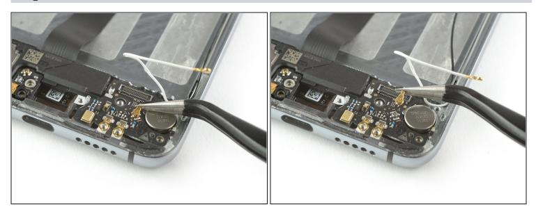
• Use a pair of tweezers to disconnect the black coax cable and fold it out of your way.
