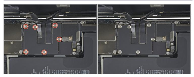
• Use a Y000 driver to remove six 1.3 mm screws securing the logic board cover bracket.
