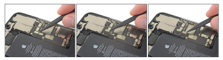
• Use a spudger or a fingernail to disconnect the Face ID dot projector and sensor cables from their sockets on the logic board.
