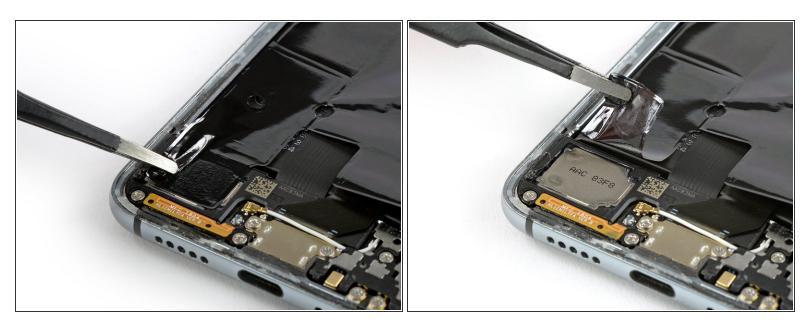
• Use a pair of tweezers to peel the black foil at the bottom end of the phone off the loudspeaker.
