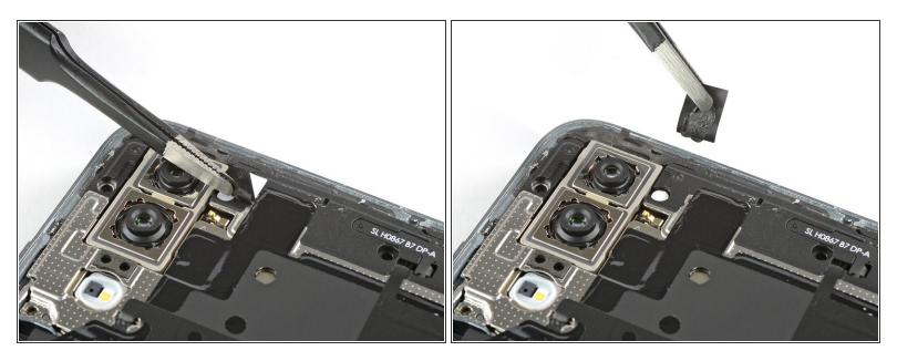
• Use a pair of tweezers to peel the black tape next to the rear camera off the motherboard cover.
