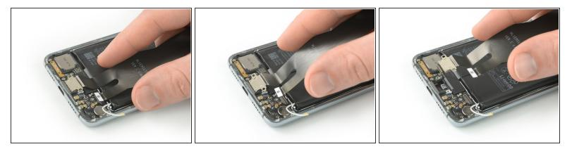
• Remove the charging port and main flex cable by lifting it upwards and then pulling it in the direction of the motherboard.
