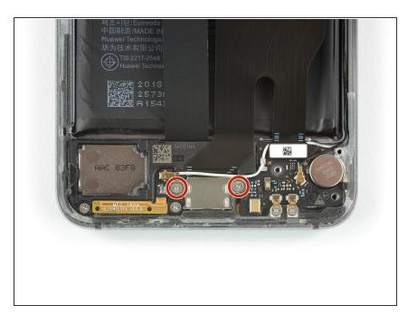
Remove the two Phillips #00 screws (3.2 mm length).
