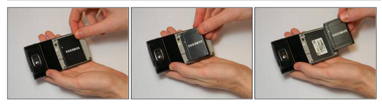
• Locate the grooves on the sides of the battery near the bottom of the phone. Use your fingers to pull the battery up and out of the phone.
