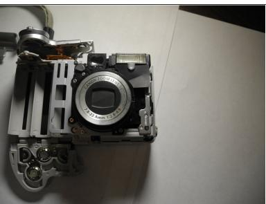
Using the pry tool, gently remove the front cover of the camera in order to expose the flash and the lens.
