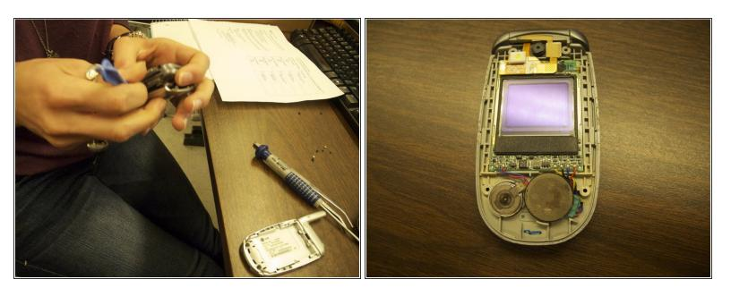
• To pry open the face plate, place the iFixit Opener tool in the crease of the phone.
