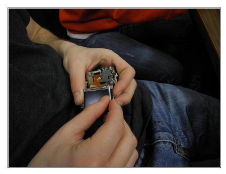
Remove outer case/rim of screen from the back of the camera. The screen should still be hanging by the red wire and white wire.
