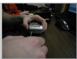
Remove the screws from the bottom, right, and left side of camera.
