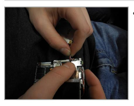
Pull out the red wire and white wire attaching the screen to the motherboard.
