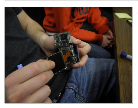
Flip up black lever holding data cable to motherboard, and remove data cable from motherboard.
