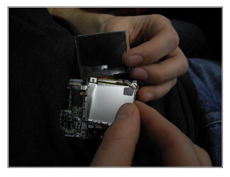
Unhinge the outer case of the screen from the back of the camera.
