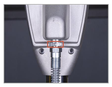
Use a 7/8" wrench to loosen the coupling securing the power cord to the handle enclosure.
