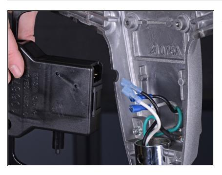
After all wires are disconnected from the interlock assembly, remove the interlock assembly from the handle.
