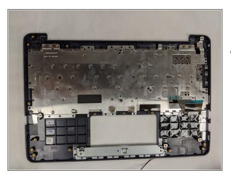
The removed keyboard assembly can be seen in this picture. As the keyboard is molded to the plastic frame of the laptop, the entire assembly must be replaced. To reassemble your device, follow these instructions in reverse order.
