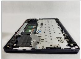
Lift the motherboard away from the computer while allowing the ribbon cable in the middle to fall through its cutout.
