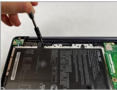
Using the Phillips #0 screwdriver, remove the two 3 mm screws located at the top and left side of the battery.
