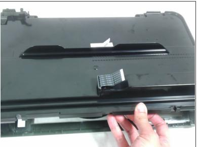
Pull the back panel towards you and lift it away from the rest of the printer cover.
