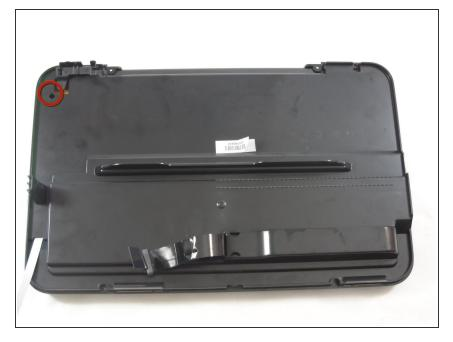
Remove one 9mm T10 Torx screw from the back of the printer lid.
