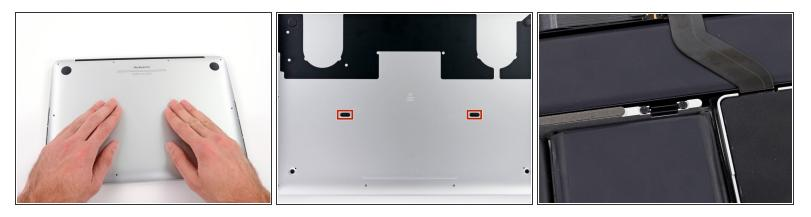
During reassembly, gently push down the center of the lower case to reattach the two plastic clips.
