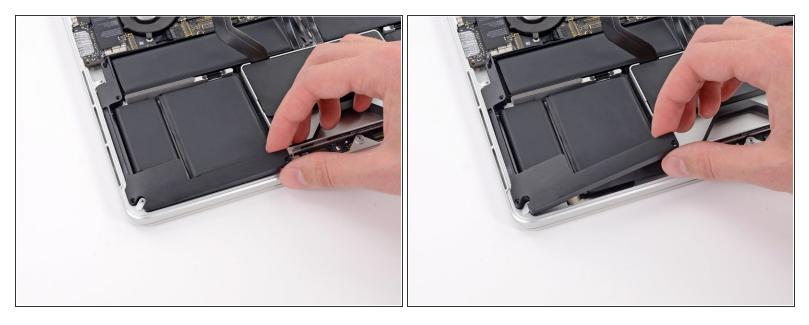
• Lift and remove the right speaker out of the upper case.
