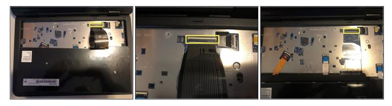
Use a plastic pry tool to lift up the plastic clip holding down the ribbon cable. Be very gentle
