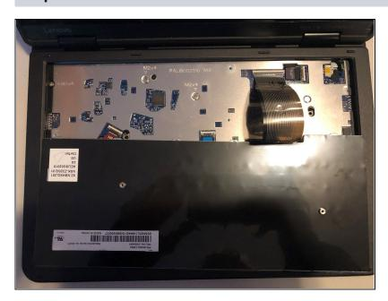
Pull slightly up from the keyboard but NOT all the way, the ribbon cable is still connected to the motherboard
