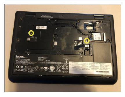
There are two screws that will need to be removed to access the keyboard.
