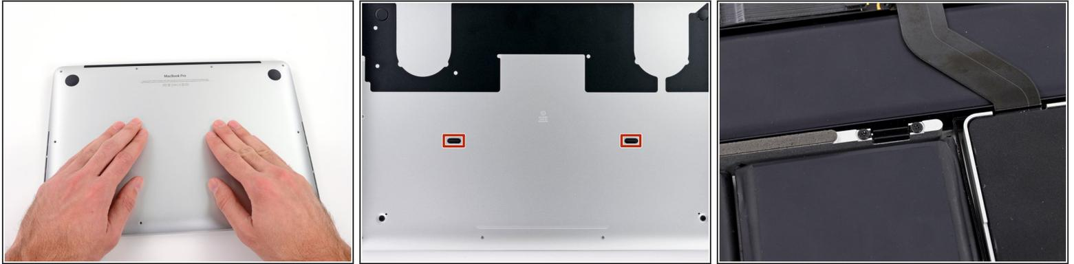
☞ During reassembly, gently push down the center of the lower case to reattach the two plastic clips.
