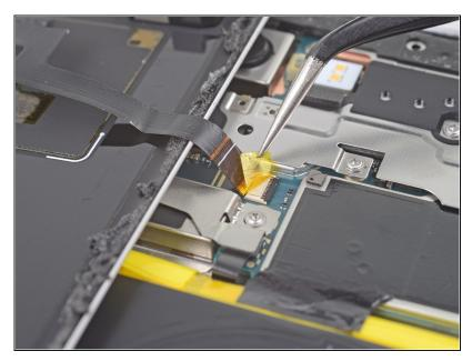
• User <u>tweezers</u> to carefully peel up the yellow tape over the fingerprint sensor connector.
