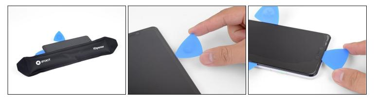
• Continue heating and slicing until you have sliced around the entire perimeter of the phone.
