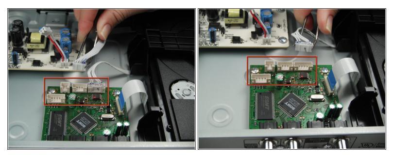
• Use the tweezers to remove the four sets of wires connected to the processing board. Start with the cord located in front of the row of three cords.
