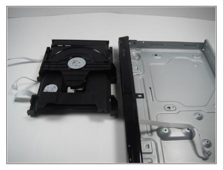
Remove the DVD drive by pulling it backward and upward while ensuring that it is free of any braces.
