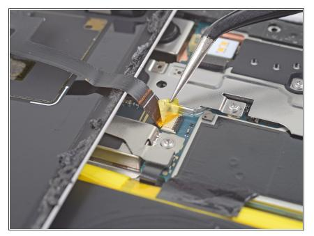
• User tweezers to carefully peel up the yellow tape over the fingerprint sensor connector.
