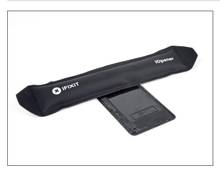
• Apply a heated iOpener over the fingerprint sensor for a minute.
