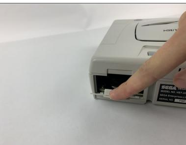
Press on the plastic lever on the back of the Sega Saturn to pop open the battery slot.
