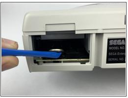
• Push up the edge of the battery with the iFixit opening tool to get the battery out of its socket.
