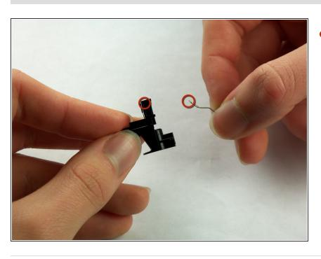
Insert the hooked section of the replacement spring into the corresponding hole on the mount.
