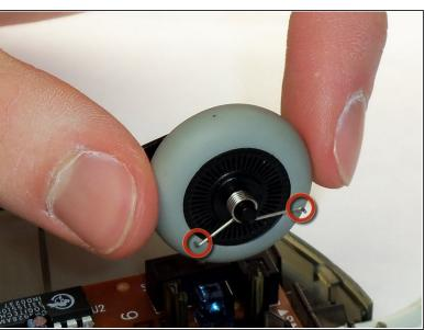
Place the replacement spring on the correct side of the wheel (shown in the images) with the prongs pointing down.
