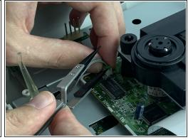
Pry the second cable out of its socket on the disk reader with the iFixit opening tool or ESD safe tweezers. When the lip of the cable gets enough distance out of the socket, it can be wiggled free.
