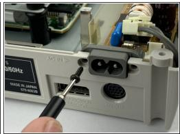
Remove the two black 11.4mm standoff screws on the back of the Sega Saturn holding the power socket in place. These screws are tight and easily stripped, so it's suggested to use a standoff screw head.
