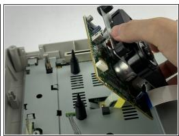
• Lift the laser reader slowly out of its slot hosted by these four pins. There is a screw underneath with a cable attached to the motherboard.
