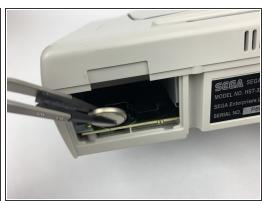
Use the ESD safe tweezers to pull the battery out of its slot.
