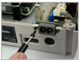
Remove the two black 11.4mm standoff screws on the back of the Sega Saturn holding the power socket in place. These screws are tight and easily stripped, so it's suggested to use a standoff screw head.
