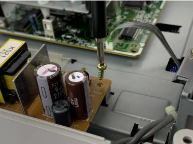
Remove the metallic 12.3mm JIS#1 screw holding down the power supply board.
