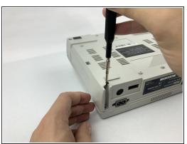
Remove the five black 13.5mm JIS#1 screws on the bottom of the device. One might be hidden by a sticker.
