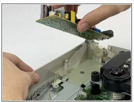
Lift the power supply board out of its socket, minding the pins that connect it to the motherboard.
