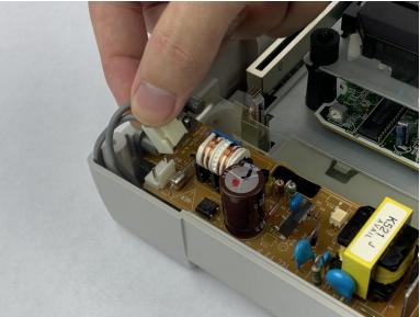
• Unplug the power button plug on the power supply board. Use the iFixit opening tool if necessary.
