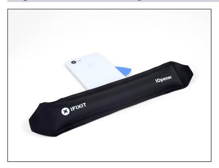
Apply a heated iOpener to the bottom of the back cover for a minute.
