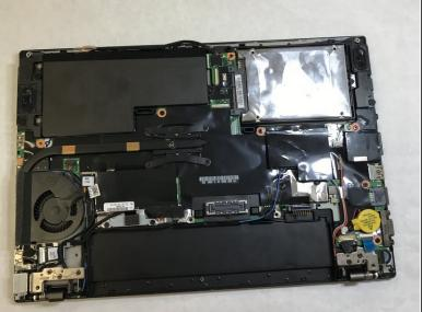
Remove the seven 5mm screws on the back cover using the Phillips #0 screwdriver.
