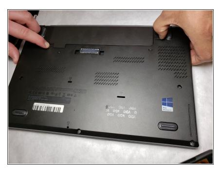
Remove the battery by pulling on the two sliding buttons next to the battery.
