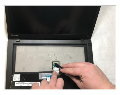
Remove the plastic covering and detach touch point and keyboard cable.
