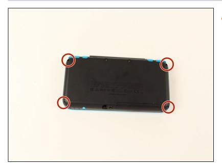
Unscrew the four 6mm tripoint screws located at the four corners of the bottom panel.
