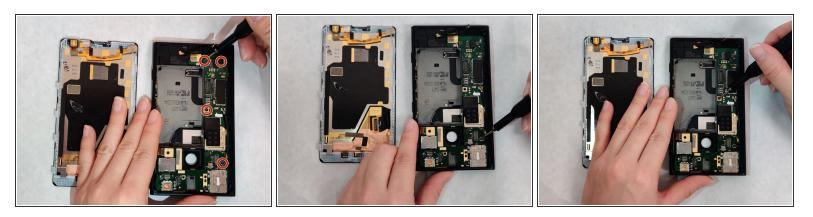
Using a T4 screwdriver, remove four 4.60 mm screws to disconnect the motherboard from the rest of the device.
