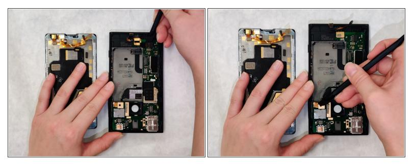
• Disconnect the two gold connectors from the motherboard using a spudger.
