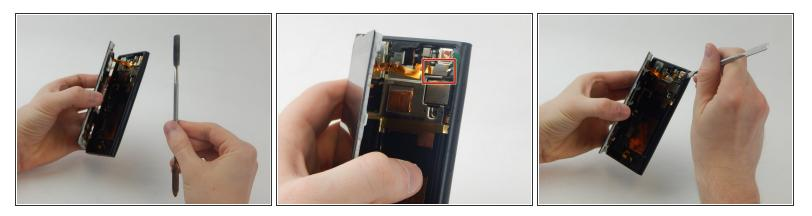
• Wedge a spudger underneath the silver rectangle in the upper right corner until it pops off the back of the phone.
