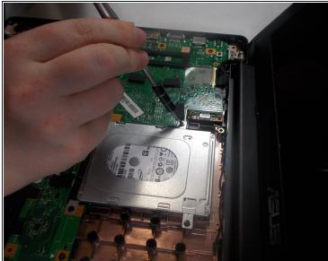
• Use a Phillips #0 screwdriver (PH0 bit) to remove the four 6.0 mm screws that are securing the hard drive.
