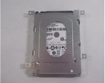
• Lift the hard drive up and pull it towards the screen so that it disconnects from the motherboard.
