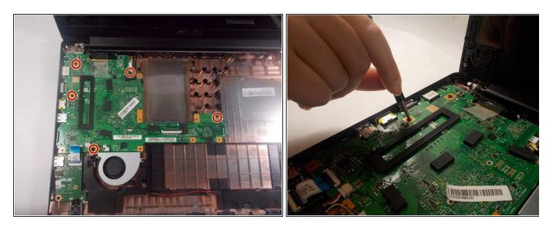
Use a Phillips #0 screwdriver (PH0 bit) to remove the five 6.0 mm screws attaching the motherboard to the base of the laptop.
