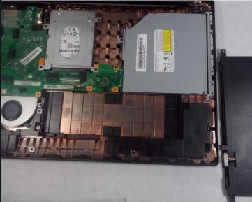
• Lift the battery up and remove it completely from the laptop.
