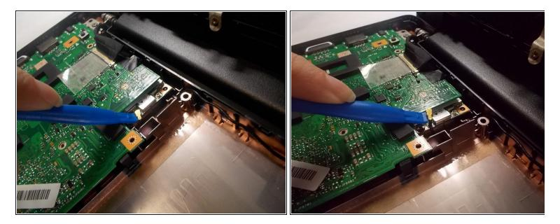
• Lift the coaxial connector from the wifi chip with the plastic iFixit opening tool.
