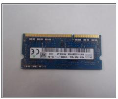
• Remove the RAM by lifting and pulling it up from the back of the motherboard.
