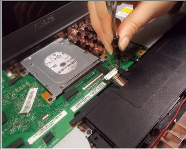
Use Phillips #0 screwdriver (PH0 bit) to remove the four 6.0 mm screws attaching the battery to the laptop.
