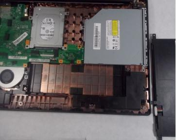
• Lift the battery up and remove it completely from the laptop.
