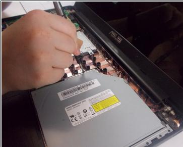
• Use a Phillips #0 screwdriver (PH0 bit) to remove the one 6.0 mm screw holding in the optical drive.
