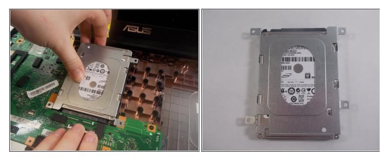
• Lift the hard drive up and pull it towards the screen so that it disconnects from the motherboard.
