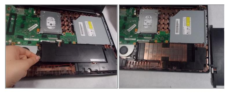
• Lift the battery up and remove it completely from the laptop.
