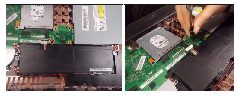
Use Phillips #0 screwdriver (PH0 bit) to remove the four 6.0 mm screws attaching the battery to the laptop.
