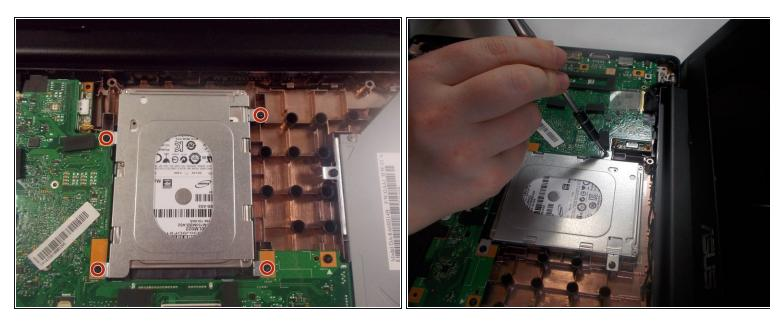
• Use a Phillips #0 screwdriver (PH0 bit) to remove the four 6.0 mm screws that are securing the hard drive.
