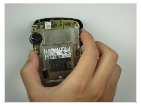
• With one side loosened, simply lift the phone internals to separate from the front casing.
