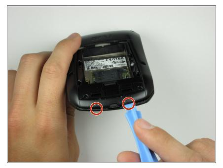
Use the plastic opening tool to apply pressure on the two clips that are located at the bottom of the phone.
