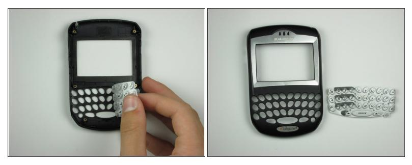
• Peel off the rubber keypad buttons from the face plate.
