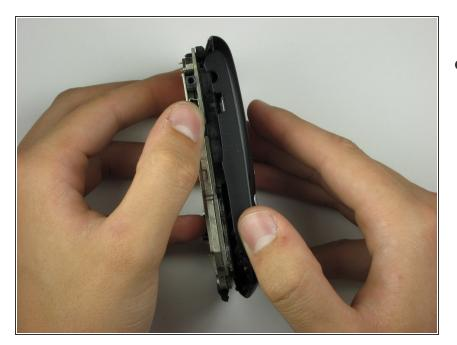
To remove the phone's internals, start by loosening one side by pulling gently.
