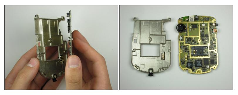
• Separate the logic board mounting plate from the logic board by lifting with minimal force.
