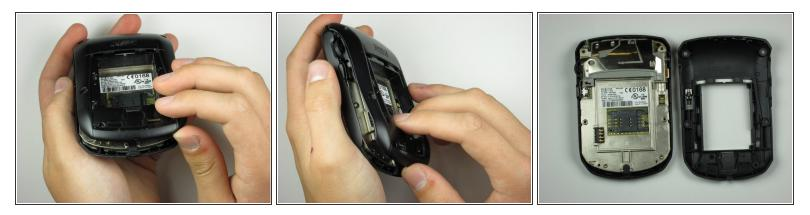
• Remove the back casing from the phone by lifting the unhooked portion, then slide the casing towards the top of the device.
