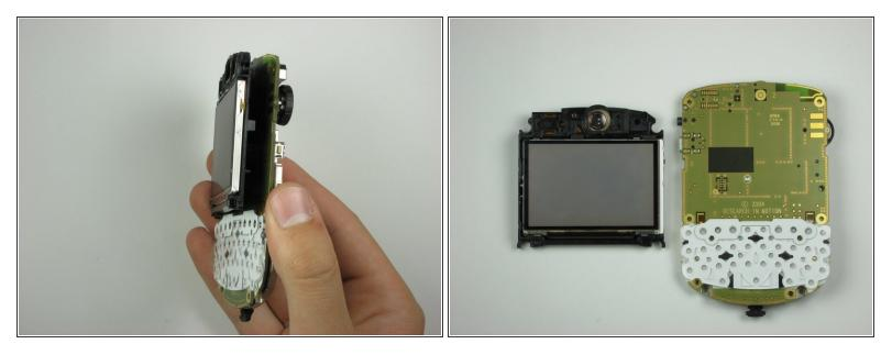
• With the clip unhooked, gently separate the display from the phone internals by pulling.
