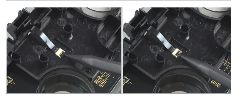
Use a spudger to flip up the locking tab on the ZIF connector.
