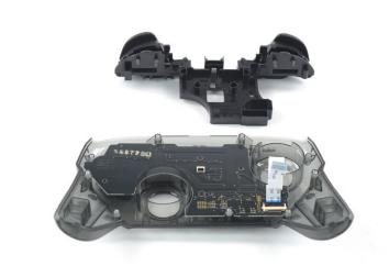
Remove the trigger buttons from the plastic cover.
