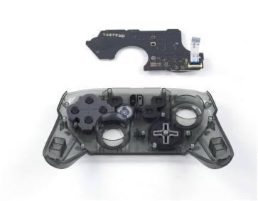
Remove the circuit board.
