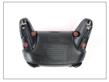
Use a JIS #00 screwdriver to remove the four silver 6.8 mm screws that secure the clear back plastic cover.
