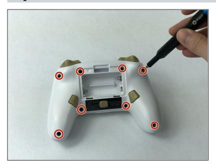
Remove all eight screws using the J0 screwdriver.
