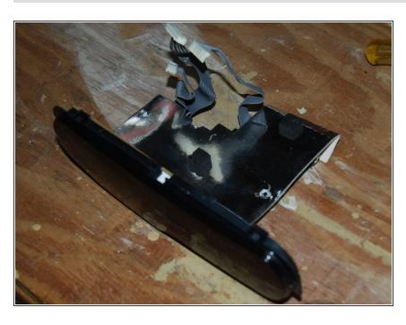
Pull display cover and display board away from bottom shell and set aside.
