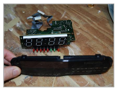
Separate the display cover from the display board.
