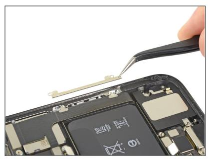
• Remove the flex cable bracket.
