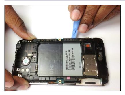
• Insert the plastic opening tool between the rear inner frame and the motherboard and slowly work your way around the device.
