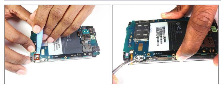
• Using the tip of an plastic opening tool flip up the tab holding the capacitive button ribbon cable.
