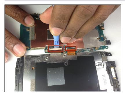
• Using the plastic opening tool pop up the two tabs connecting the LCD and motherboard.
