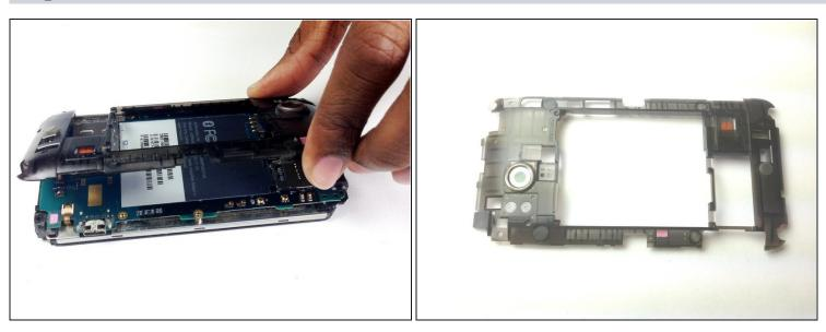
• Remove the rear inner frame from the rest of the device.
