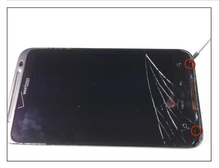
• Remove the two Phillips screws where the plastic cover was.
