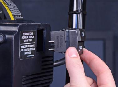
Remove the power switch from the electrical box.
