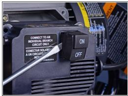
Use a flathead screwdriver or a pry tool to pry the power switch away from the electrical box.
