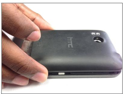
• Lift and remove the rear panel.
