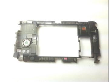
• Remove the rear inner frame from the rest of the device.
