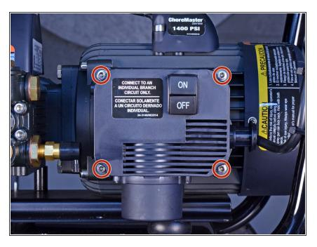
Remove the four 59.2 mm-long 4 mm hex socket bolts from the electrical box.
