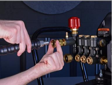
i Disconnect all hoses and unplug the power cord before performing any repairs on the Mi-T-M electric pressure washer.
