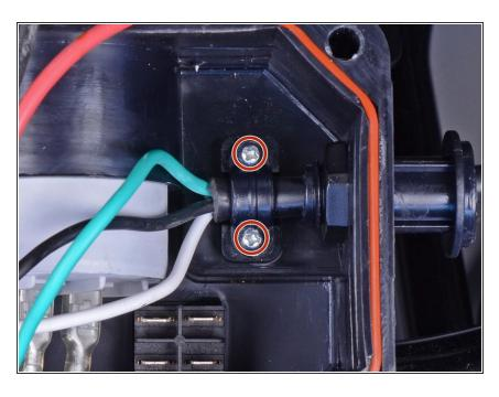
Remove the two Phillips screws securing the power cord strain relief bracket.
