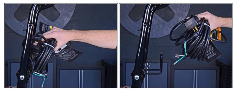
Remove the power cord from the pressure washer.
