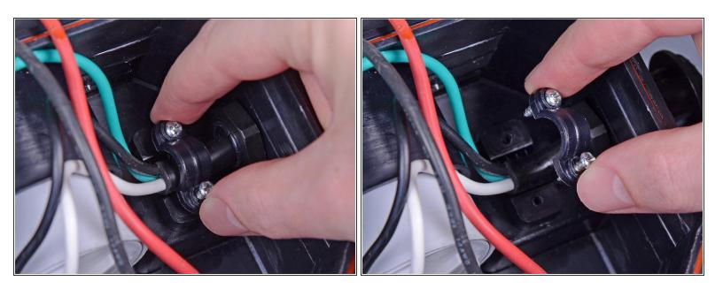
Remove the power cord strain relief bracket.
