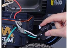
Remove the three wire ends of the power cord from the electrical box.
