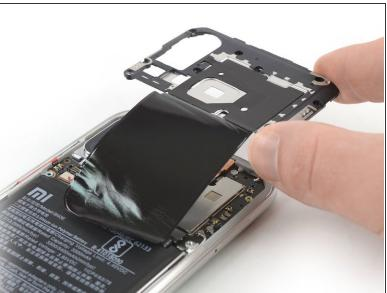
Carefully remove the motherboard cover including the NFC antenna.
