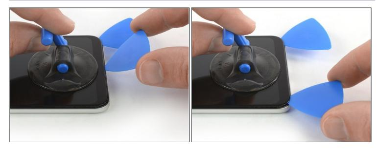
• Insert the tip of a second opening pick and slide it to the bottom left corner of the Xiaomi Mi 8 to cut the adhesive. Leave it there to prevent the adhesive from resealing.
