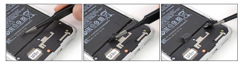
• Use a pair of tweezers to peel the black ends of the adhesive tabs off the battery.
