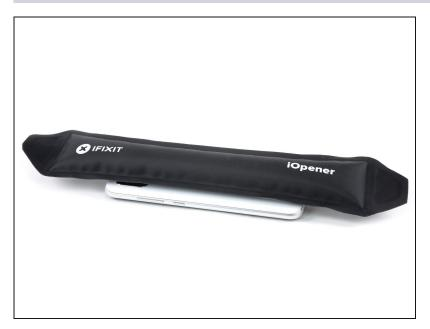
Apply a <u>heated iOpener</u> to the rear glass to loosen the adhesive beneath the edges. Apply the iOpener for at least two minutes.
