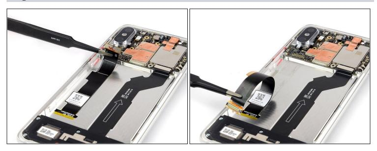
• Use a pair of tweezers to peel the display flex cable off the midframe. It is attached with mild adhesive.
