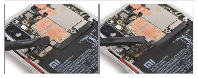
• Use a spudger to pry up and disconnect the battery flex cable located at the bottom of the motherboard.
