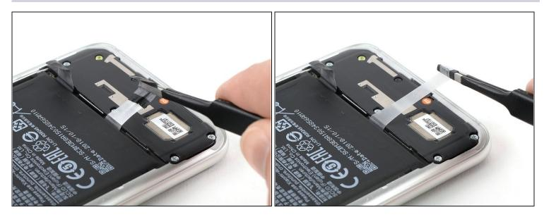
• Pull out the first adhesive tab from underneath the battery.
