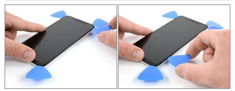
• Insert the tip of a fifth opening pick at the top right corner of the phone and slide it along the right edge to cut the adhesive.
