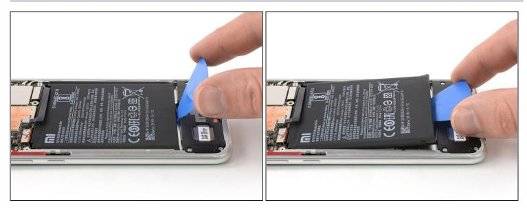
• Use an opening pick or plastic card to pry the battery out of its recess until you can get a good grip.
