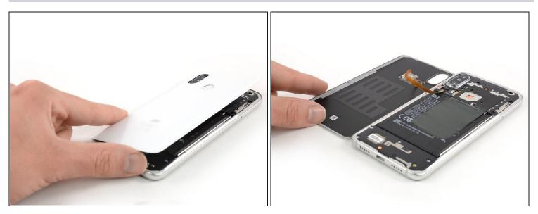
• Carefully lift the rear glass and fold it to the left side to access the fingerprint flex connector.
