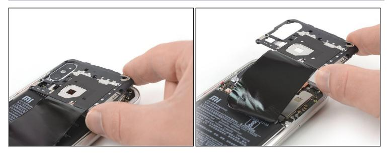
• Carefully remove the motherboard cover including the NFC antenna.
