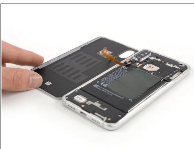
Carefully lift the rear glass and fold it to the left side to access the fingerprint flex connector.
