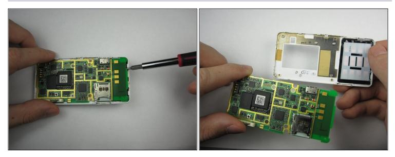
• Carefully pry the motherboard off of the back case
